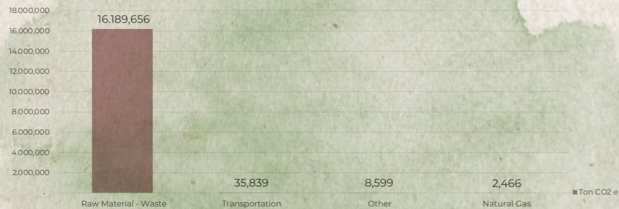
Graph 25. Emission Distribution according to Spinning Factory Classes *Other: Emissions from air conditioning, refrigerator losses/leaks, generator, product packaging products and fire extinguishers
